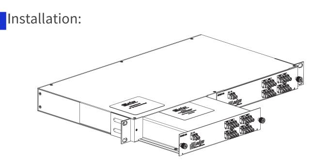
In order to install CWDM LGX Module in 19" rack, please order 19" 1U sub-rack supporting up to two LGX modules. Product code LGX-RCK-2-1U.
